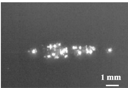
FIG. 2. An image of the bubble cloud taken by a high speed camera. The bubble cloud was generated by a single pulse of three cycles in gas saturated free water. It was used for the laser beam alignment. The ultrasound pulse propagated from the left to the right side of the image.
